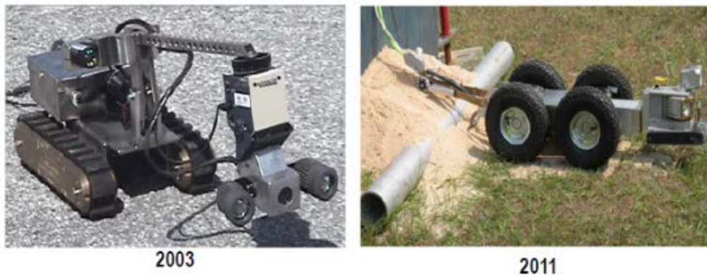
Fig. 7. Two of five different robots developed for the H-Canyon Exhaust Tunnel at Savannah River [1].
