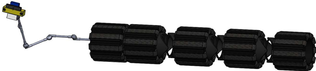
Fig. 9. MOTHERSHIP with 5 modules, 3 articulating joints, 1 rigid joint and extended arm with sensor package.
