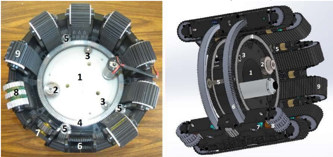
Fig. 2. Close-up view of the 2-D tread module, highlighting the gear arrangement.
