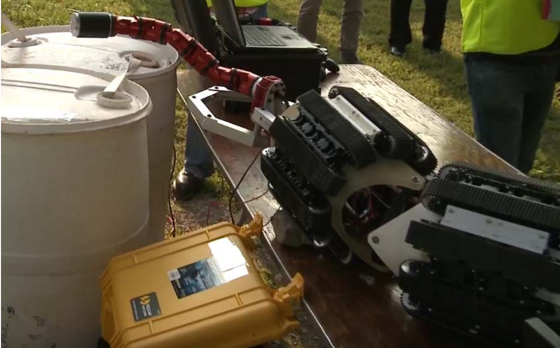
Fig. 6. A modular snake robot attached to the MOTHERSHIP through an X-module base. A camera module with laser range sensor is attached as an end effector to demonstrate highly articulated inspection tasks at the Portsmouth Gaseous Diffusion Plant.
